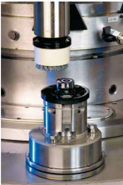
Consolidated machining of injection parts (defined edge deburring) with force controlled deburring brush
