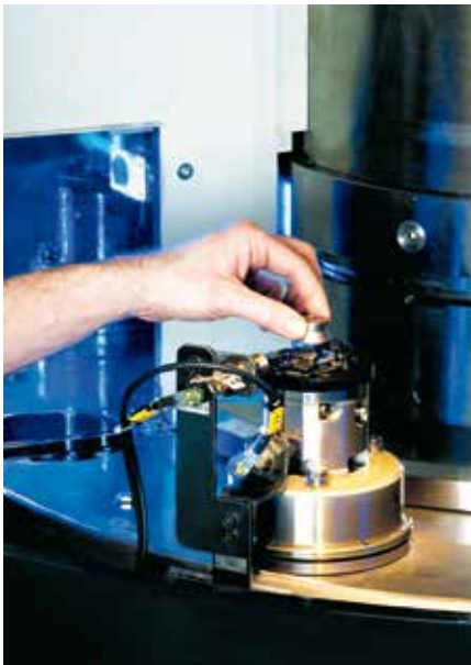
Hand loading with light curtain and automatic switch off
