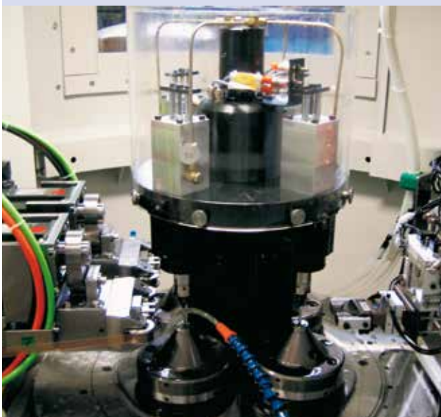
Machining of needles with diamond tape
