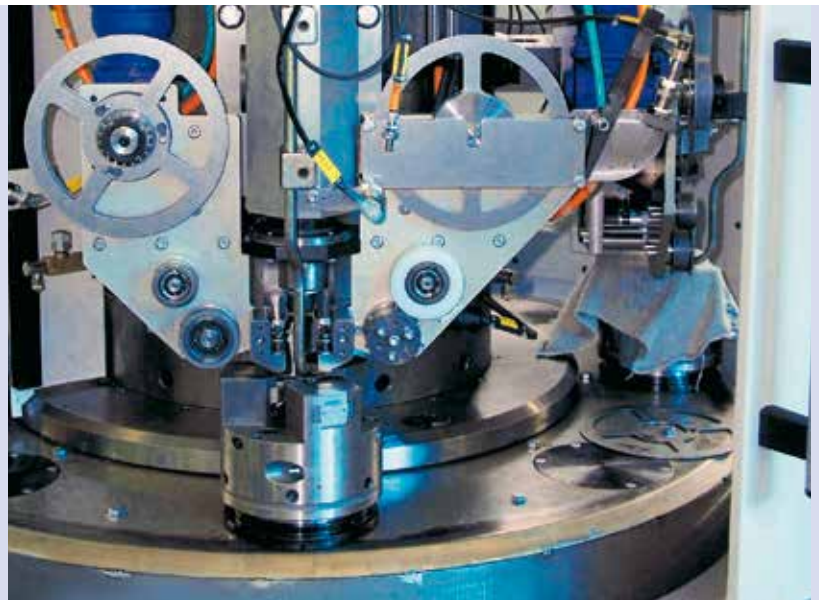
Patented consolidated machining of injection parts (sealing seat machining) with tape
