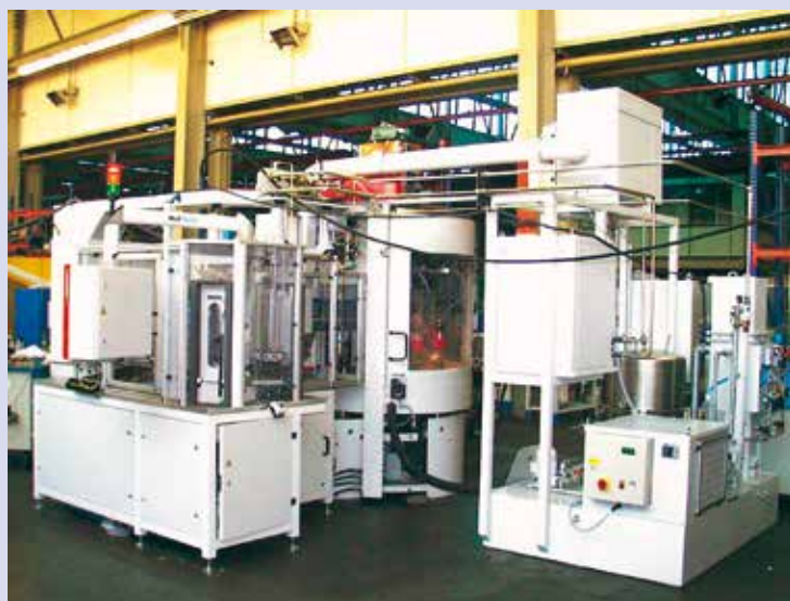
MicroStar with automation cell; bulk container into staple grid with pre- and in-process gauge as well as with SPC unit
