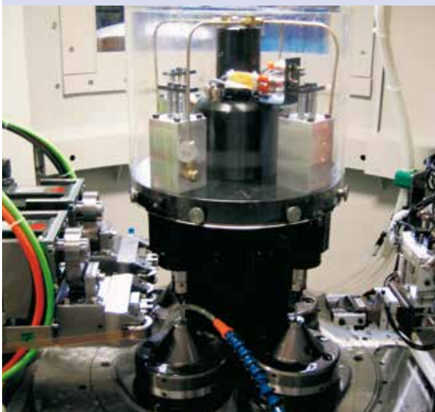
Machining of needles with diamond tape
