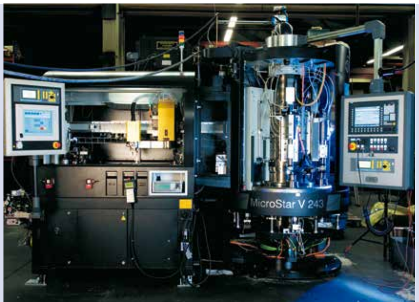
MicroStar with automation and integrated pin insertion unit for injection parts
