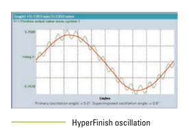
Primary oscillation angle: ± 5.0°. Superimposed oscillation angle: ± 0.8°
