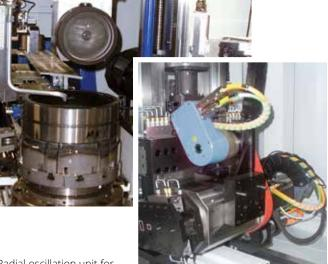
Radial oscillation unit for roller bearing inner rings
