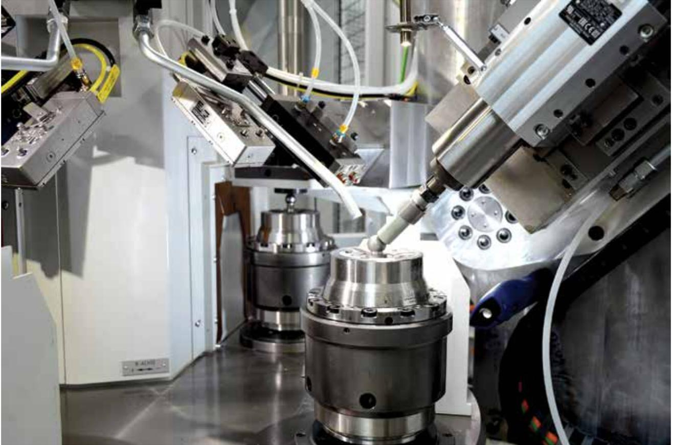
The SpheroStar has two tool spindle units that can automatically rotate by up to 90 degrees so that the optimal machining position for the relevant process is always selected.
